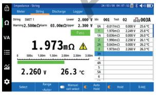
Discharge testing: measure cell impedance, voltage, and temperature.
