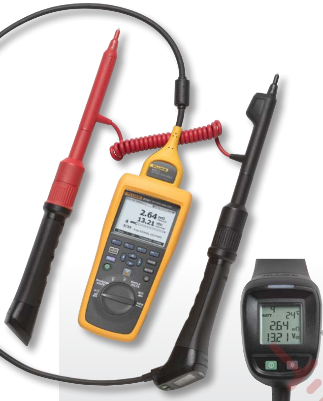
Intelligent test probe with integrated LCD display
