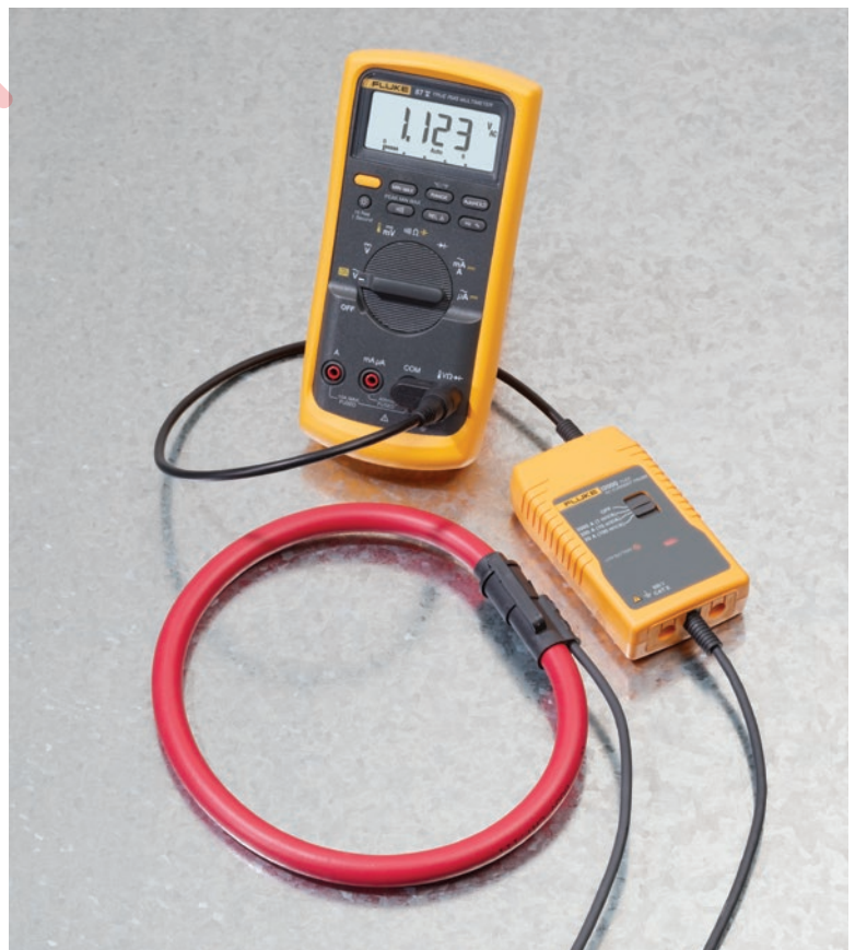
i2000 Flex connected to a Fluke 87V Digital Multimeter.
