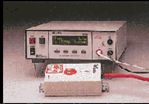
Hypot II shown with standard remote receptacle box for testing products terminated in a line cord.
