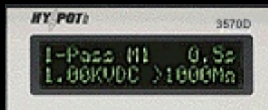
Display shows a pass condition for an insulation resistance test.
