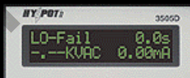
Display shows a LO-fail condition on a AC withstand test. Minimum current not met.
