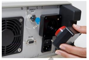
As an option, the  $973-SF_6$  is now available with integrated, industry standard chemical-based  $SO_2$ measurement – another indicator of potential problems within gas-insulated equipment. The measurement cell is conveniently located on the rear panel for easy user replacement when needed (about every two years). Low cost, precalibrated, interchangeable modules make this swap-out a simple, two minute field operation.
