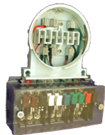
(CA000579) TTS-13 Temporary Test Switch for 6S and 9S meters ---- This allows you to remove a socket meter, plug in the adapter with the test switch and then plug the meter into the adapter for 6S and 9S meters.
