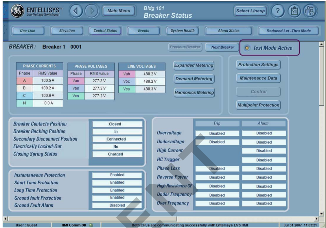
Figure 2-2 HMI screen showing circuit breaker in Test Mode
